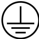
Figure 4. Equipment Earth (Ground) Point
